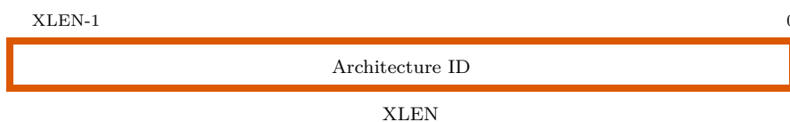
Figure 1.3: Machine Architecture ID Register ( marchid ).
