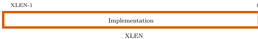
Figure 1.4: Machine Implementation ID Register ( mimpid ).
