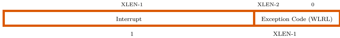
Figure 1.8: Machine Cause Register ( mcause ).
