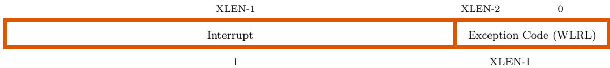
Figure 1.8: Machine Cause Register ( mcause ).
