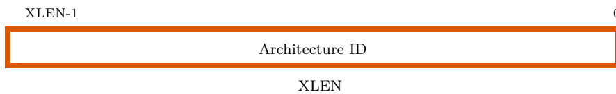
Figure 1.3: Machine Architecture ID Register ( marchid ).
