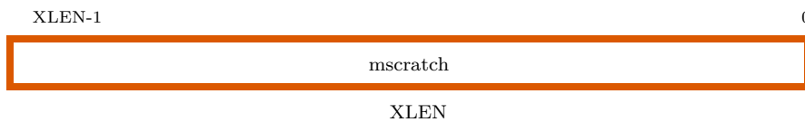
Figure 1.14: Machine-mode scratch Register ( mscratch ).
