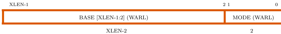
Figure 1.9: Machine Trap-Vector Base-Address Register ( mtvec )
