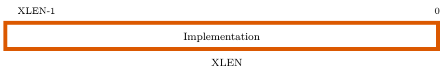
Figure 1.4: Machine Implementation ID Register ( mimpid ).
